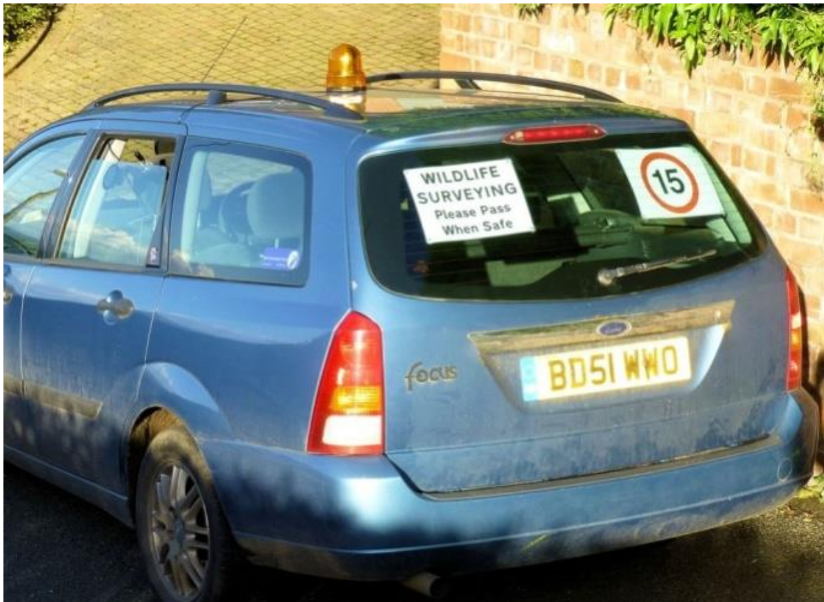
Figure 14: An example of a car ready to carry out a driven transect. The bat detector microphone is positioned just inside the open car window to avoid wind noise.
